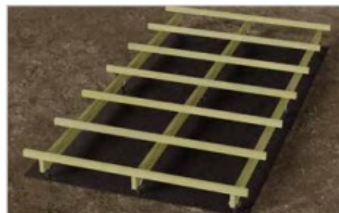
Example for a cross-wood structure with joists of 45x145 mm and bearers of 45x70 mm
