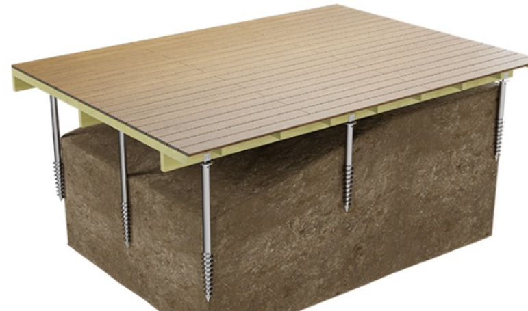
Step 4: Placing the planks
