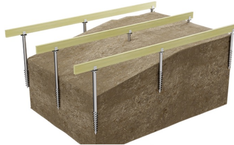
Step 2: Placing the joists
