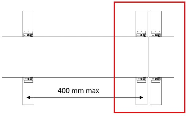
Double joisting at the ends of the boards
