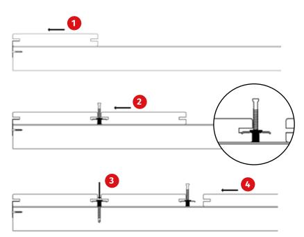
**1.** Fitting the Start/End clip, then laying the first board
