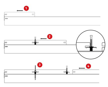
**1.** Fitting the Start/End clip, then laying the first board
