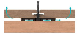
The Airspacer wedge promotes ventilation between the board and the joist without affecting clip functionality or wood movement.
